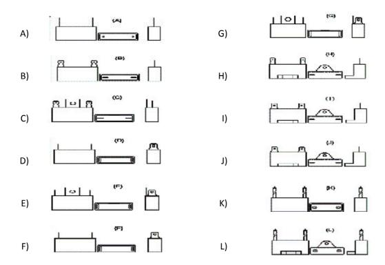
**Integral mounting ear**: Many type CBB61 capacitors have integral mounting ears. This ear makes it an excellent choice for difficult to mount applications and the choice of terminal configurations is another big plus.
