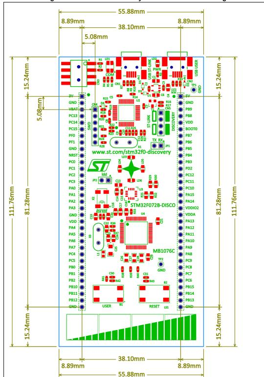
Figure 8. STM32F072 Discovery board mechanical drawing
