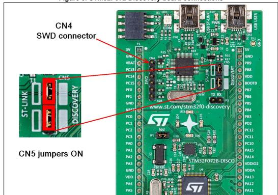
Figure 5. STM32F072 Discovery board connections
